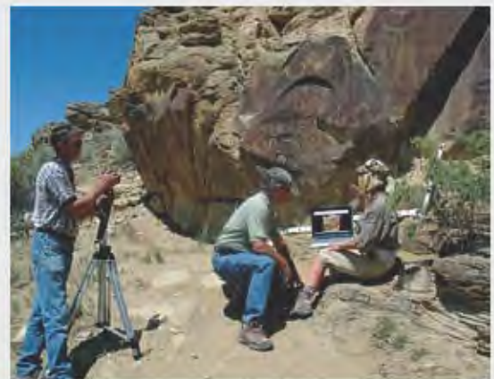
Figure 18. The close-range photogrammetric digital 3D image models can be created and viewed on a laptop computer in the field, providing an on-site demonstration.
